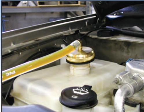
Removal of coolant through surge tank.
