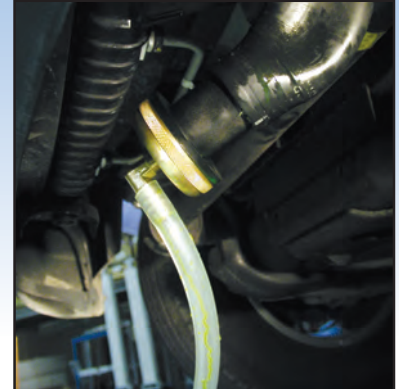
Removing coolant from engine heads by pulling a vacuum. This prevents coolant from mixing with and contaminating oil in cylinders.
