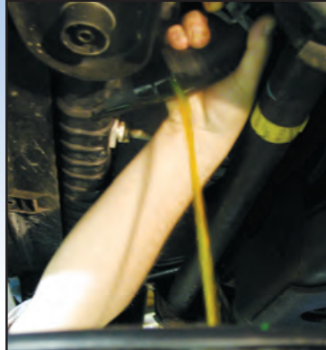
Controlled release through lower radiator hose while pulling vacuum at top of system.
